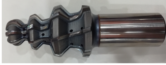
Figure 1: A complex cutting tool whose meridian contains several points of only C^0 continuity.
